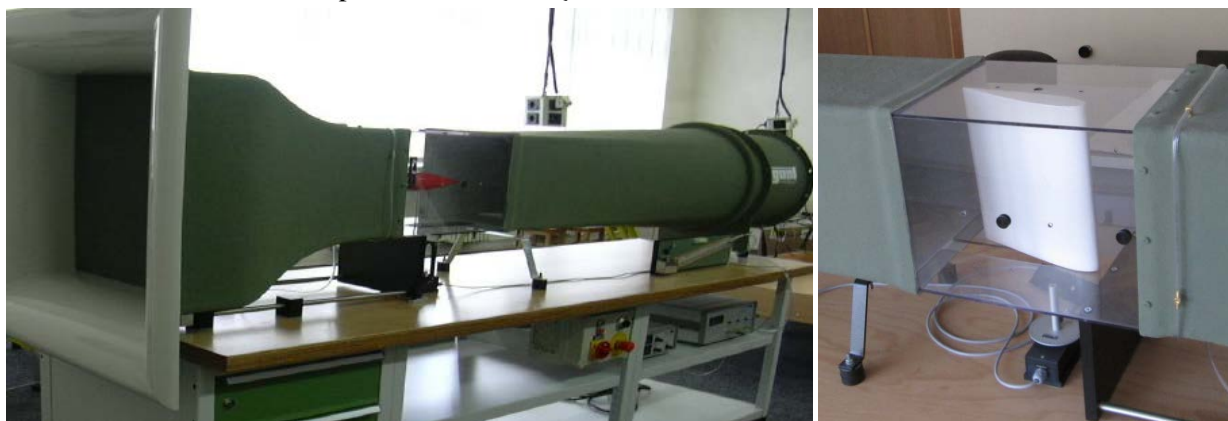
Figura 2.2.1 Tunel aerodinamic subsonic GUNT Model experimental supus cercetării
